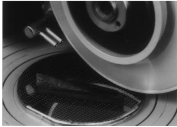
Titanium carbide bars diced with a nickel blade Figure 1
